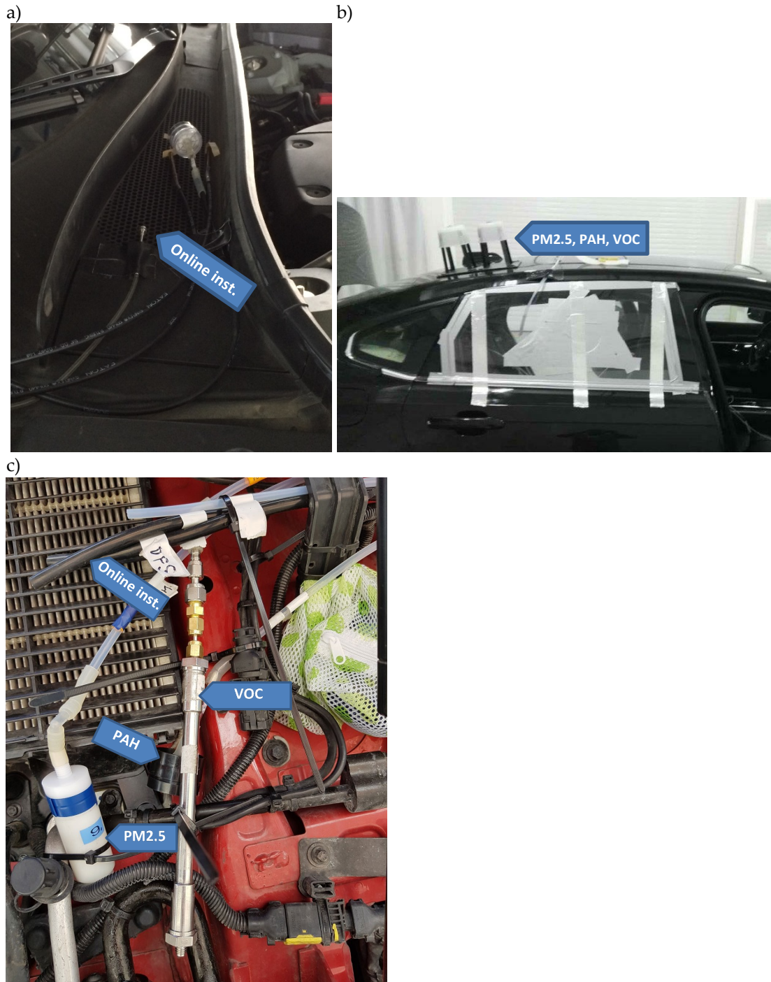
Figure A1. Inlet for the outside air samples a) for the online particle instrument in the passenger car, b) for the pumped samples in the passenger car (the front of the car in a and b is to the right), c) for all sampling of the outside air in the truck.
